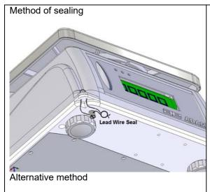
The scale has got metallic loops on the base and the cover, located at the right rear corner as shown here. A metal pin or wire can be passed through the loops and sealed using a lead-wire seal. Ensure the seal is secured enough to prevent removing the cover without breaking the seal or damaging the enclosure.
