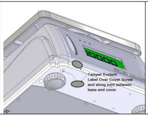
An alternative method would be to use tamper-evident labels over the screw on the bottom cover and over the joint between the top and the bottom cover as shown in the adjacent figure.
